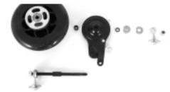
Fig 21 & 22. Pull the old wheel out. Note the arrangement of the hardware sequence. The spacer order is small, medium, large, with the small spacer between the brake and frame, the medium between the brake and wheel, and the long between the wheel and frame (refer to following sequence).
